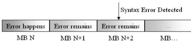
Fig. 2. Illustration of error detection lag, yielding error detection at an incorrect (macro-) block.
