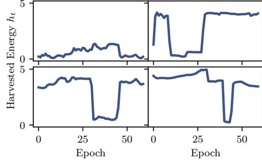
Fig. 4: Harvested energy with respect to epoch under four different instances. They follow different patterns and deviate from the i.i.d. assumption.
