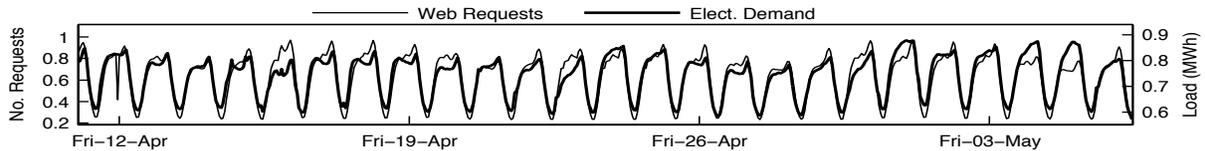
Figure 3: Evolution of the (aggregated) electricity demand and web workload between April 12th and May 6th 2013.
