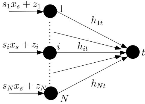
Fig. 3. A subnetwork of general layered network with  $L$  relay layers, depicting  $l^{\text{th}}$  layer with  $N$  relay nodes and a node in the  $l+1^{\text{st}}$  layer. The received signal component at node  $i$ ,  $1 \leq i \leq N$ , in the  $l^{\text{th}}$  layer is denoted as  $s_i x_s$ , where  $x_s$  is the source symbol and the corresponding noise component is denoted as  $z_i$ .
