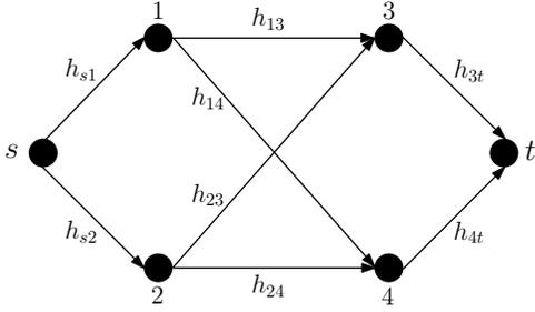
Fig. 4. General layered network with 2 relay layers between source  $s$  and destination  $t$ . Each layer contains two relay nodes.
