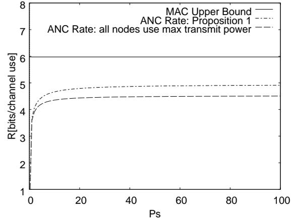
Fig. 5. Comparison of the ANC rate achievable with the scheme in Proposition 2 with the MAC upper bound for the layered network in Figure 4 with  $P_1 = P_2 = P_3 = P_4 = 10, h_{14} = h_{24} = 2$  and all other channel gains are equal to 10. Also plotted is the ANC rate when the scaling factors for all relay nodes are set to their respective upper-bounds.
